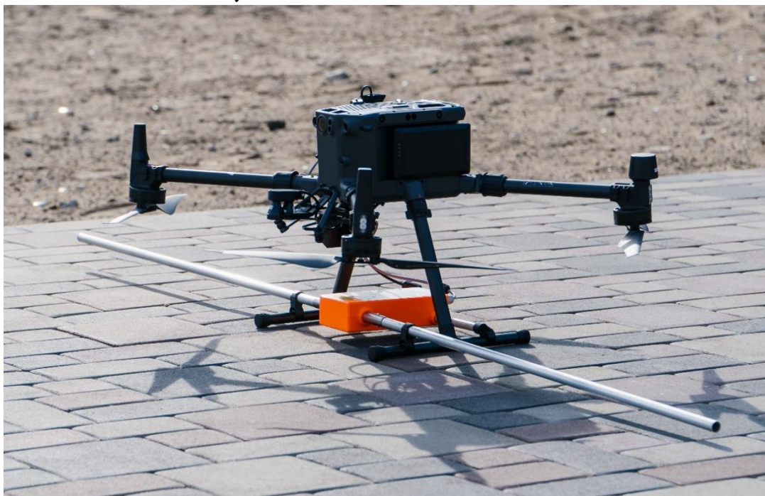
Zond Aero LF GPR system mounted on DJI M300 RTK drone:
